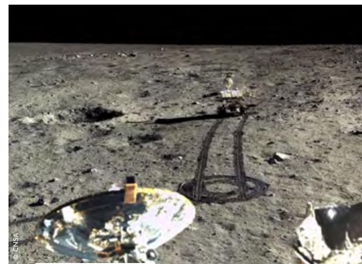
// LA SONDE CHINOISE CHANG'E 3 A DÉPOSÉ LE ROVER LAPIN DE JADE (YUTU) SUR LA LUNE EN 2013. LES DEUX ENGIN NOUS TRANSMETTENT ENCORE DES INFORMATIONS SUR LE VIEILLISSEMENT DE LEURS COMPOSANTS DANS L'ENVIRONNEMENT LUNAIRE (VIDE ET TEMPÉRATURES EXTRÊMES).
